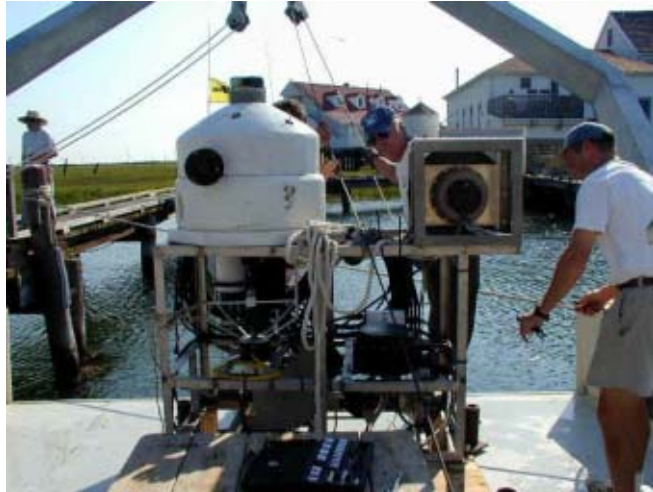
Figure 2. Profiler used in study. Instrument cage is on left and winch on the right of the profiler.
